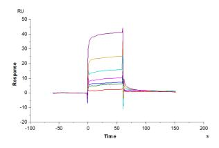
Human PGLYRP1, hFc Tag captured on CM5 Chip via Protein A can bind Human TREM1, His Tag with an affinity constant of 17.39  $\mu$ M as determined in SPR assay (Biacore T200).
